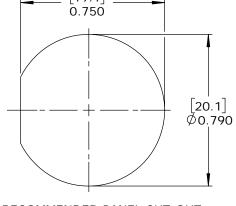
**RECOMMENDED PANEL CUT-OUT** TOLERANCE ±.003 [0.08]
