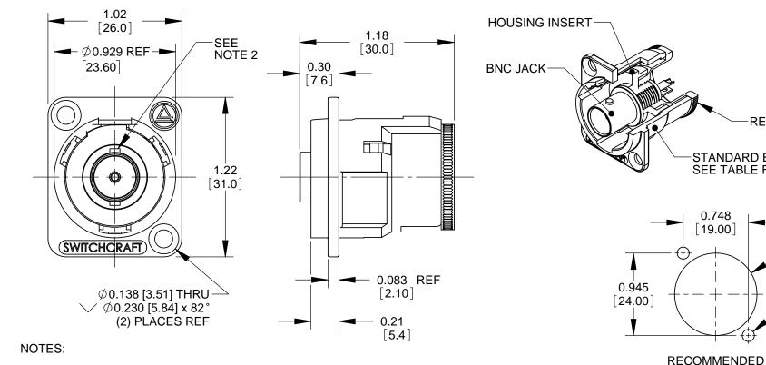
1. MATERIALS: **HOUSING - ZINC ALLOY** HOUSING INSERT - THERMOPLASTIC, BLACK RETAINING NUT - COPPER ALLOY, NICKEL PLATED BNC JACK - COPPER ALLOY, NICKEL PLATED
