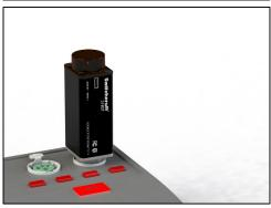
318BT can be connected directly to any XLR input (MIC Level), but before connecting; it is a good practice to ensure the Phantom Power is turned OFF on the input jack where 318BT is to be connected.
