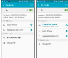
After 30 sec, both Red and Yellow LEDs will blink, this means the device is ready to be paired, turn on the Bluetooth connectivity on your device (Phone, PC, tablet ...etc.) and connect to the 318BT with the name **Switchcraft 318BT**.
